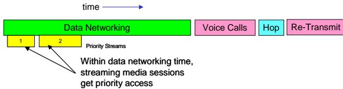
**Figure 10: Principles of the HomeRF Priority Asynchronous Data Mechanism**
