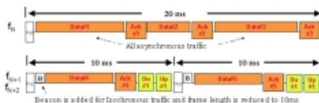
**Figure 6: HomeRF frame structure both with, and without, active voice connections (Not to scale)**
