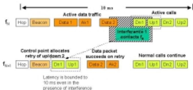
**Figure 7: HomeRF provides a unique mechanism to retry voice packets**
